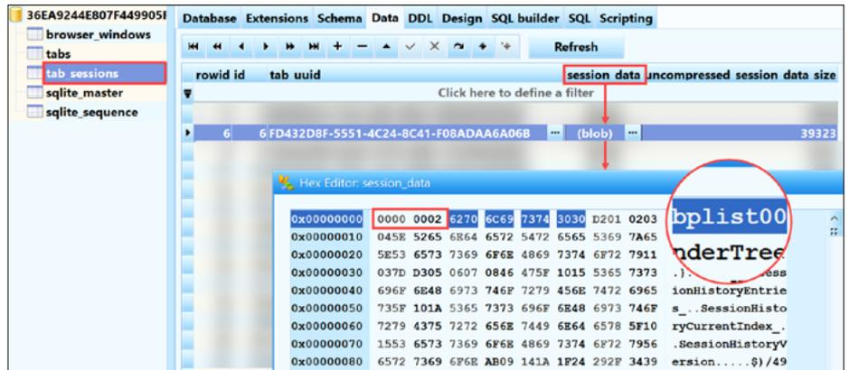
Figure 5: Apple binary property list with a four-byte offset from the start of data
